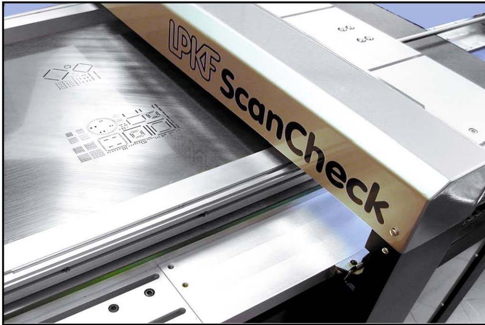
MicroScreen's LPKF AOI compares the total aperture count from the scanned data to the original Gerber data. The aperture total would also identify extra apertures and pinholes caused by debris in the chemical etching process. Sometimes laser cut apertures are cut through but are not extracted properly and are hung up in the aperture. Similarly, a chemically etched stencil with a deformed aperture caused by resist residue would also be identified.
